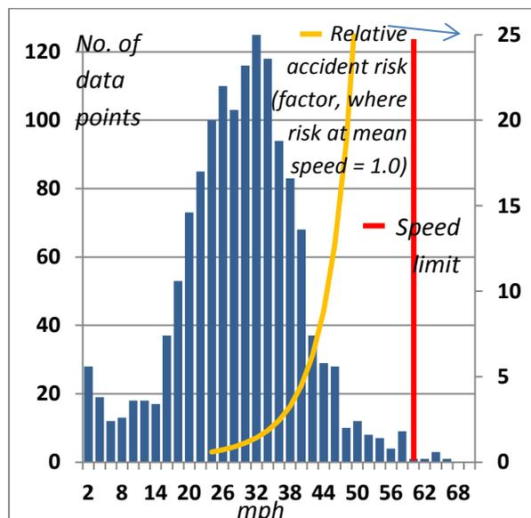
**Figure 5** (left) shows the distribution data that the SafeSpeed database holds for this short stretch of road, together with the speed limit and the relative accident risk (right hand scale), calculated in accordance with the exponential relationship discussed in the first part of this paper, and based on the mean speed of approximately 30mph for the distribution.
