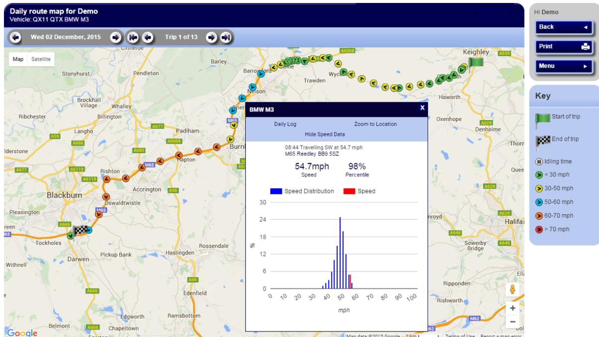
Each data point can be selected individually, providing both a clear view of the speed distributions of other drivers on the road and the vehicle being tracked, which in this case is on the 98<sup>th</sup> percentile.
